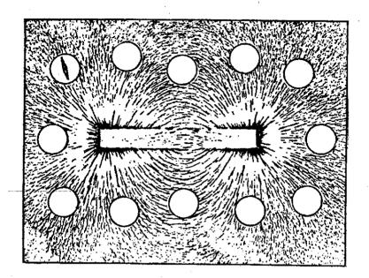
12. The illustration below is similar to Figure 36.13 (center) in your textbook. Iron filings trace out the magnetic field pattern about the loop of current-carrying wire. Draw in the compass needle orientations for all the compasses.
